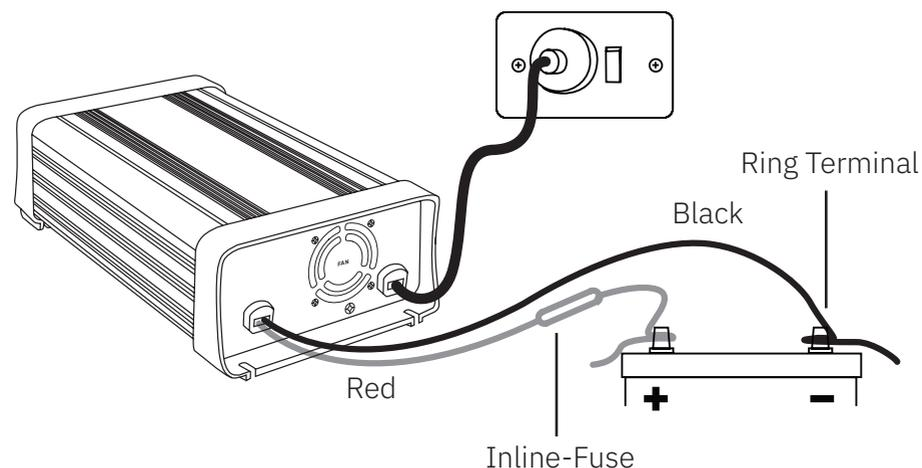
If the charger is used in a Permanent / Hard Wired application and the vehicle will not be used for some time, it is best to leave the charger connected to mains power (turned 'On') so that it can maintain the battery fully charged.
